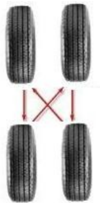
Picture 4.2-2 Tire Rotation Pattern for Front Wheel Drive Vehicle
