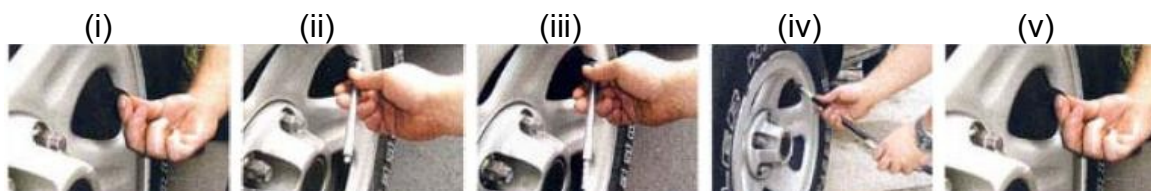
Picture 4.1 Steps in Checking Tire Pressure
