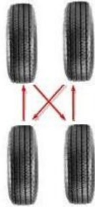
Picture 4.2-3 Tire Rotation Pattern for Rear and Four Wheel Drive Vehicle
