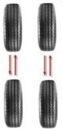
Picture 4.2-1 Correct Tire Rotation Pattern for Directional Tread
