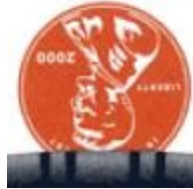
Picture 4.3 Using coin to determine if there is enough tread
