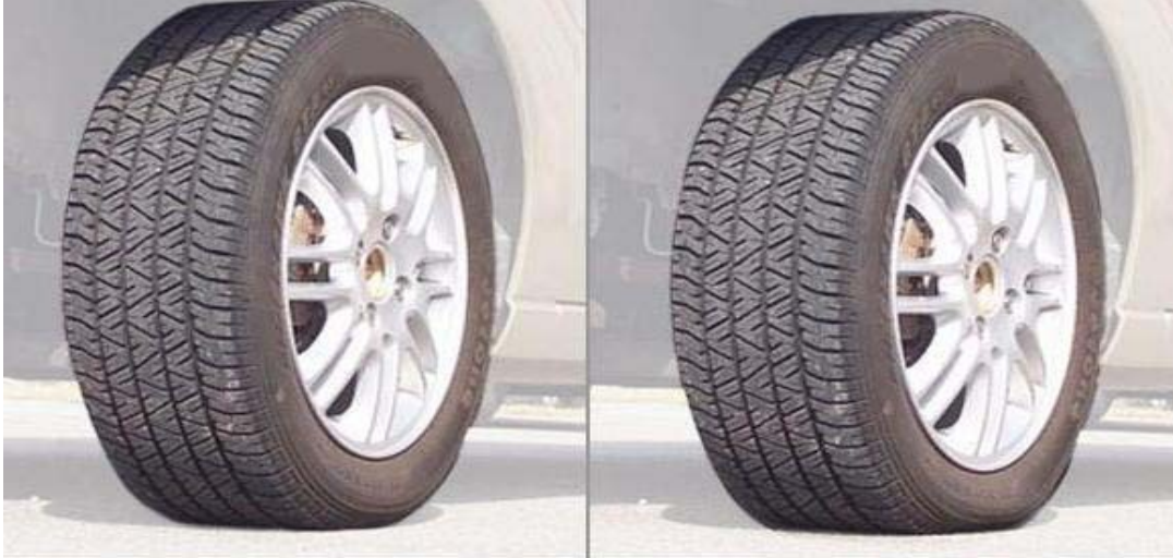
Picture 3.1 Visual comparison of 100% (left) and 50% pressure:
